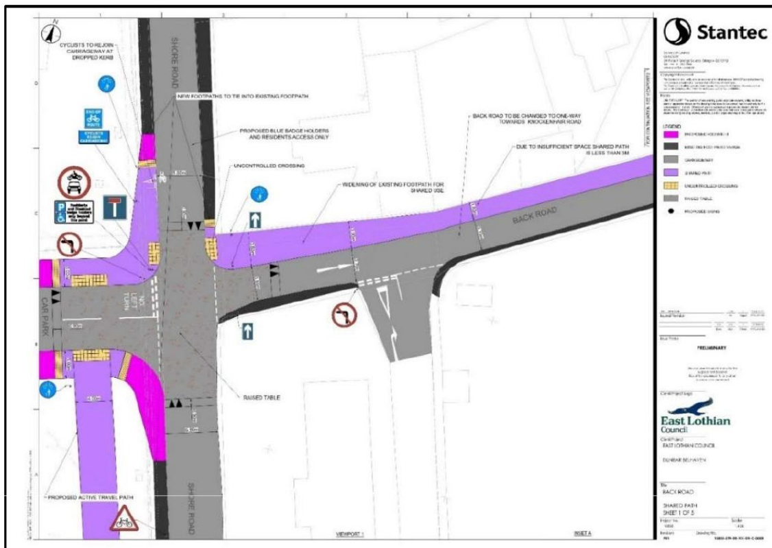
Figure 6: Improvements at Shore Road Car Park Junction (Project G)
