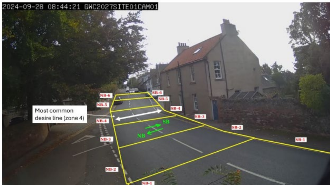
Figure 8: Diagram showing the most frequent crossing point at the Brewery Lane / High Street location
