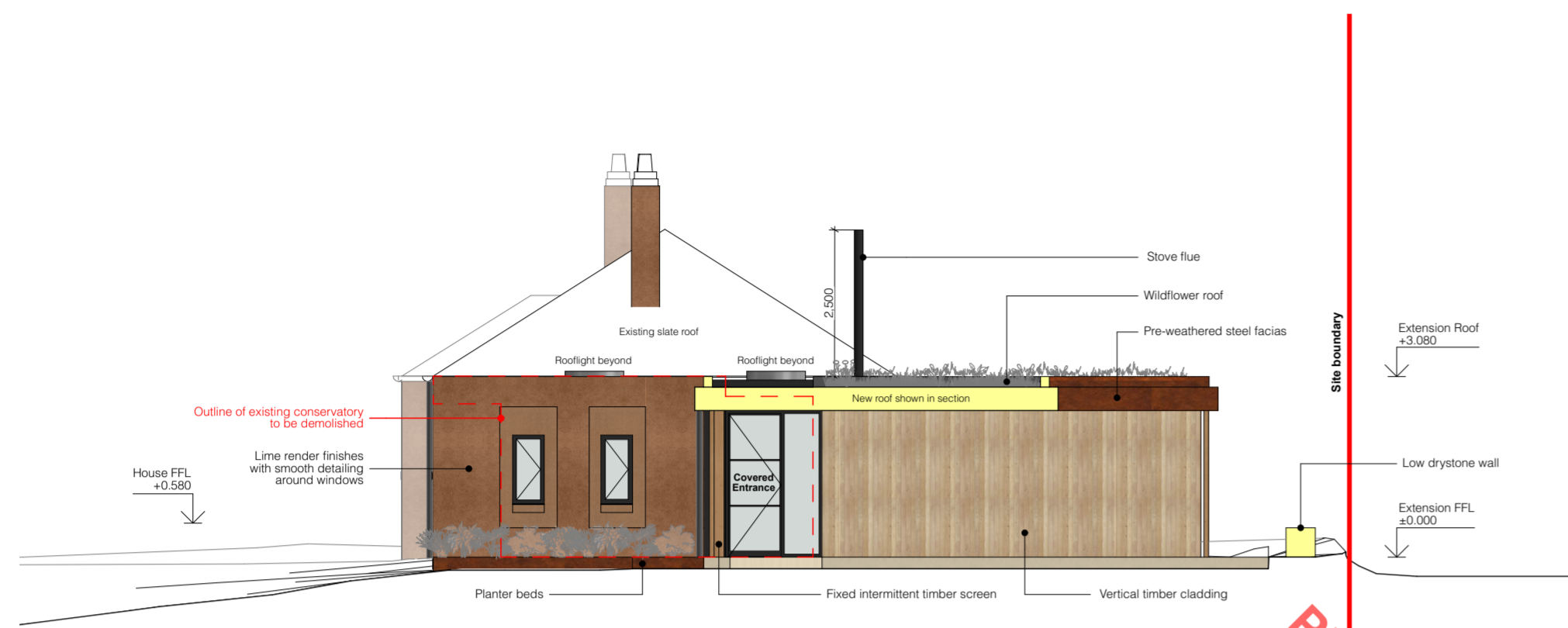
North West Elevation 1:100
