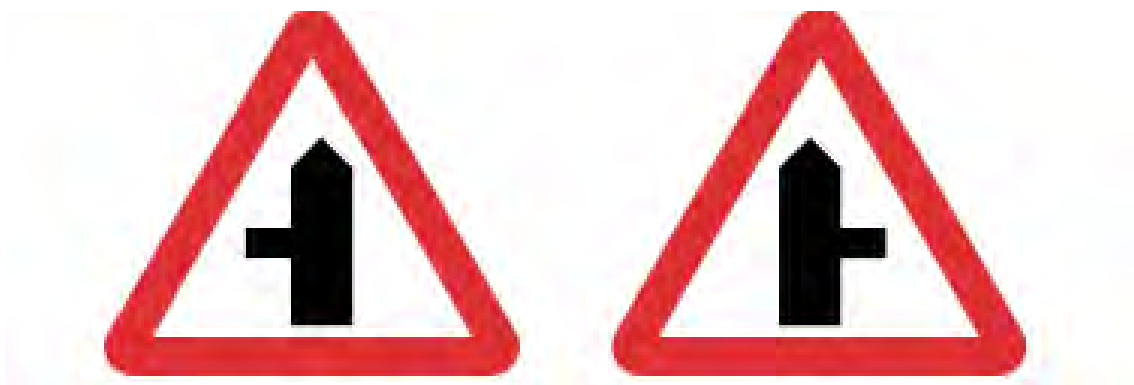
Figure 4.3 – Example of TSRGD Dia.506.1 side road ahead (Traffic Signs Manual Chapter 4)
