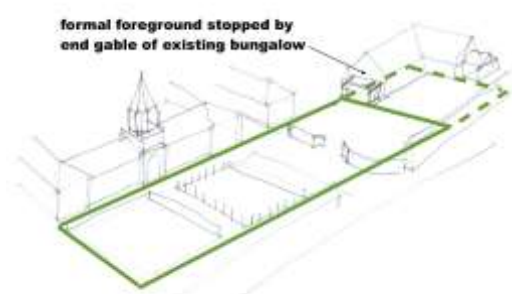
Figure 4. sketch showing how existing bungalow stops the natural extension of the formal foreground of the Listed steading
