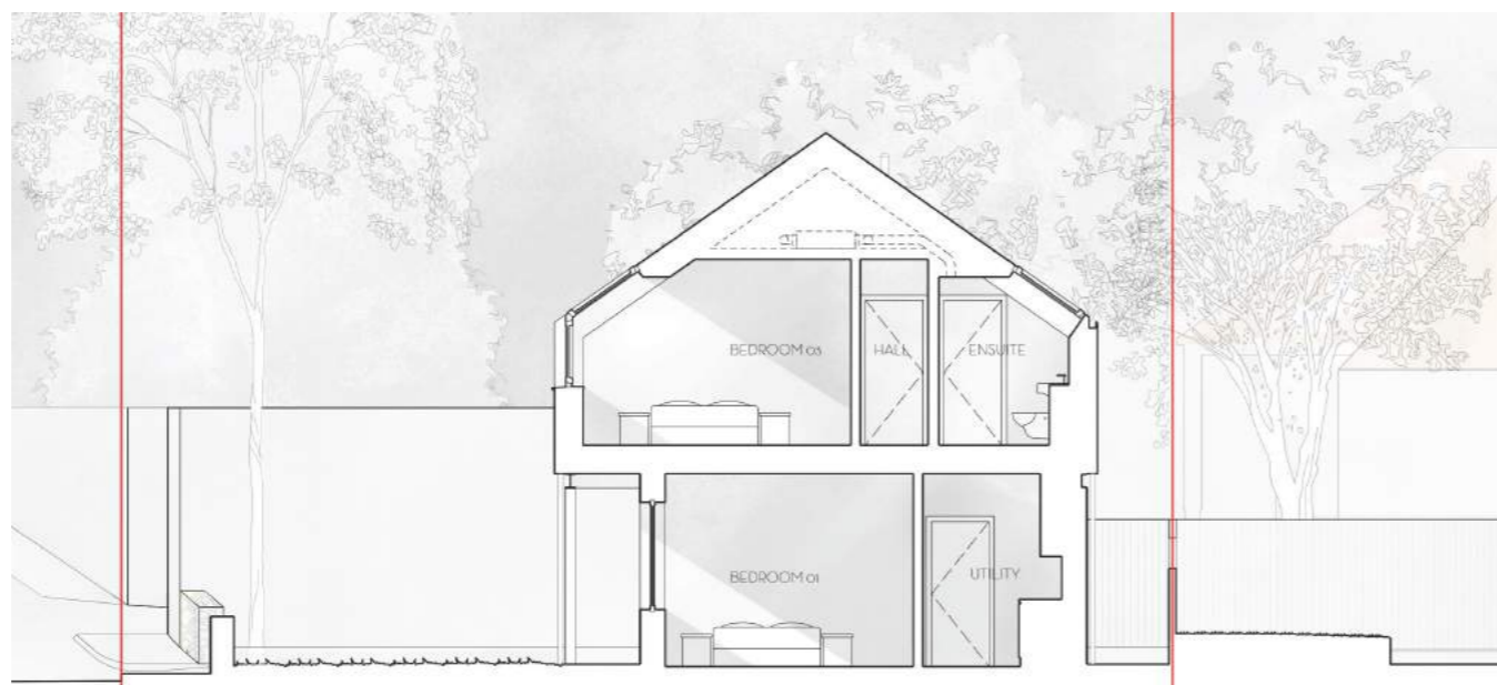
Proposed Typical Section through bedrooms, utility and en suite
