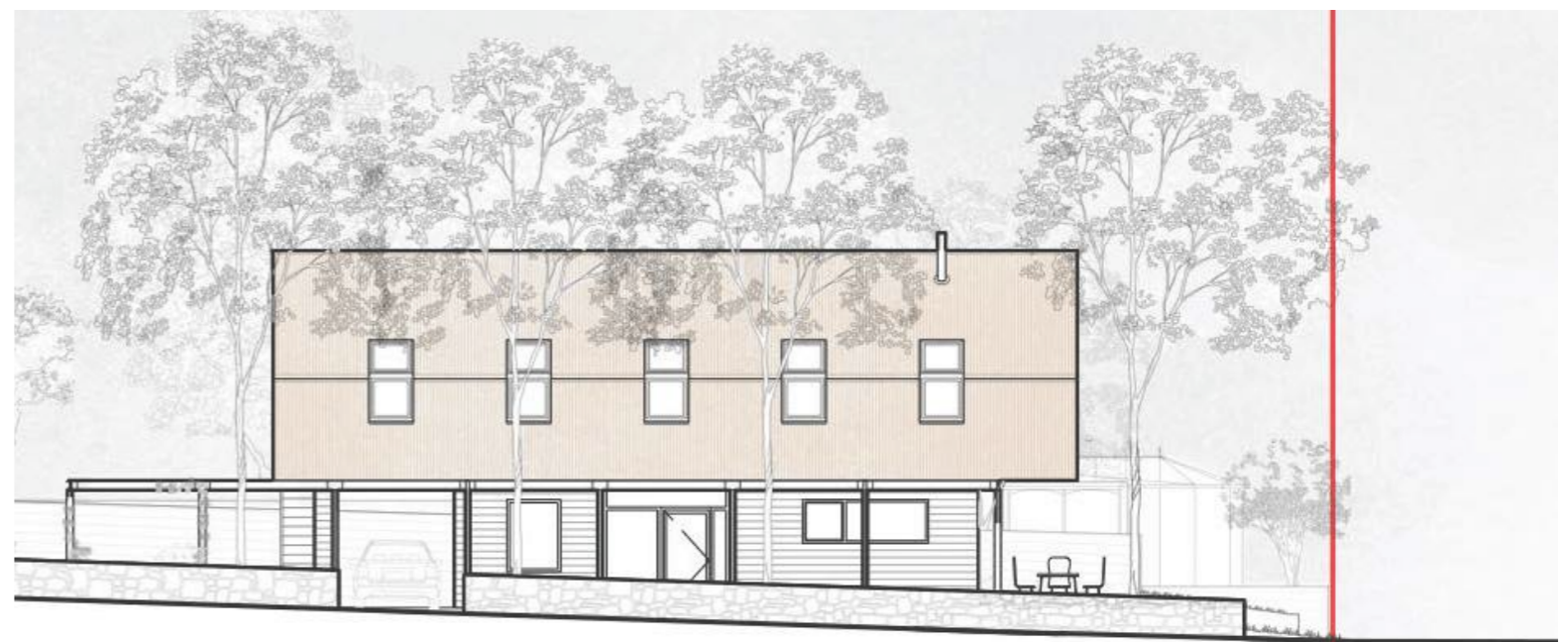
Side Elevation showing the relationship of the proposed Car Port, Colonnade, Patio and Rear Garden
