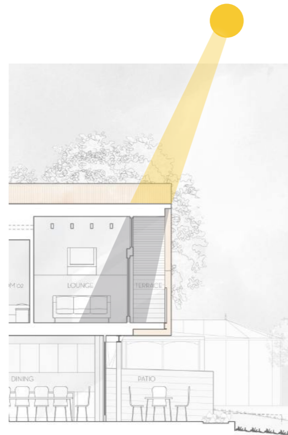
Long Section Diagram showing the protective gable, preventing overheating when the sun is at its highest in the summer
