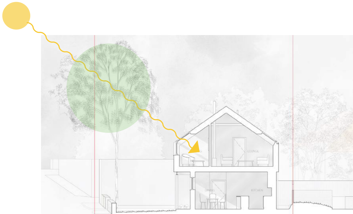
Cross Section Diagram showing the filtering effect that the trees in leaf have on the direct summer light
