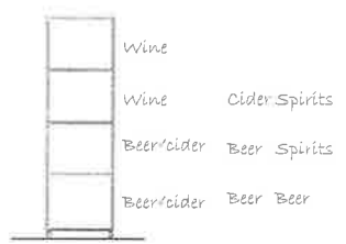
Front Elevation Refrigeration unit
