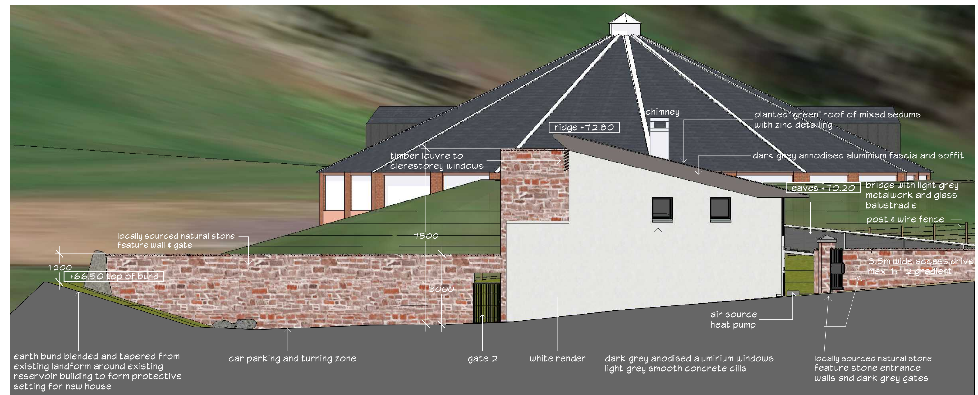
Proposed east elevation- 1:100 @ A 1
