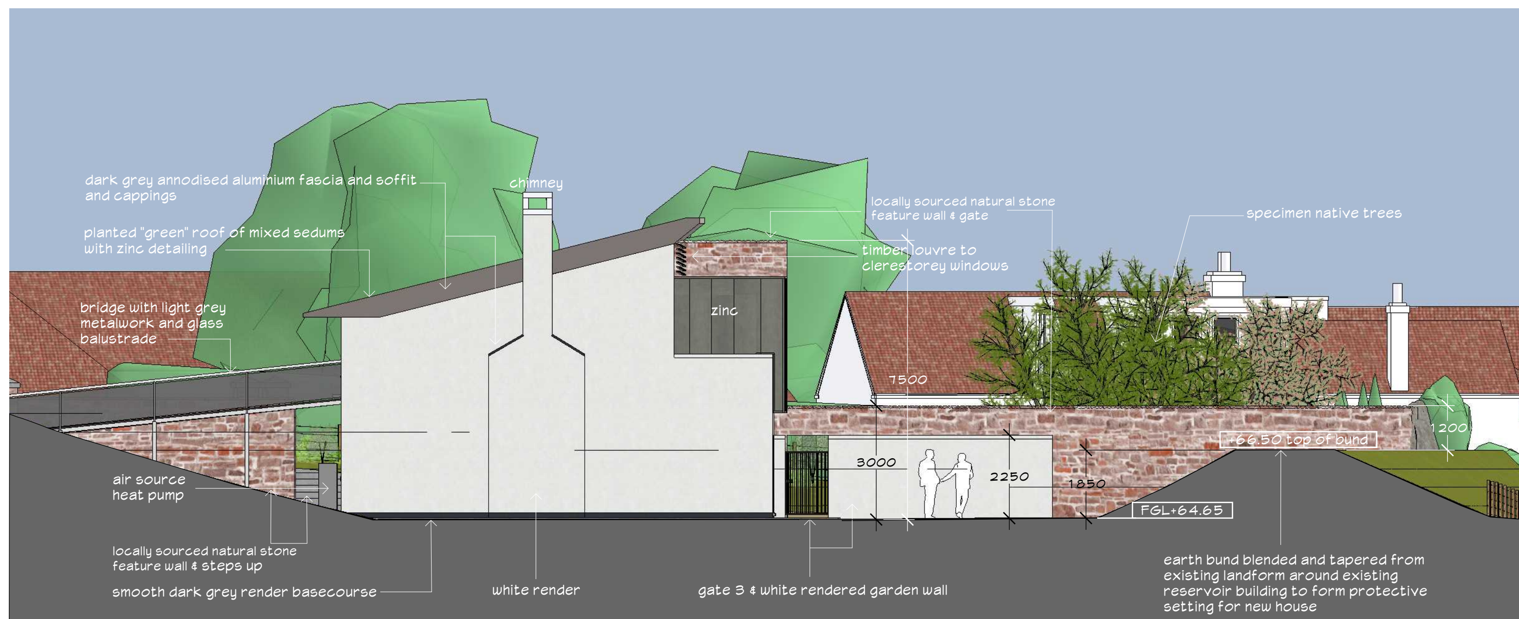
Proposed west elevation- 1:100 @ A 1
