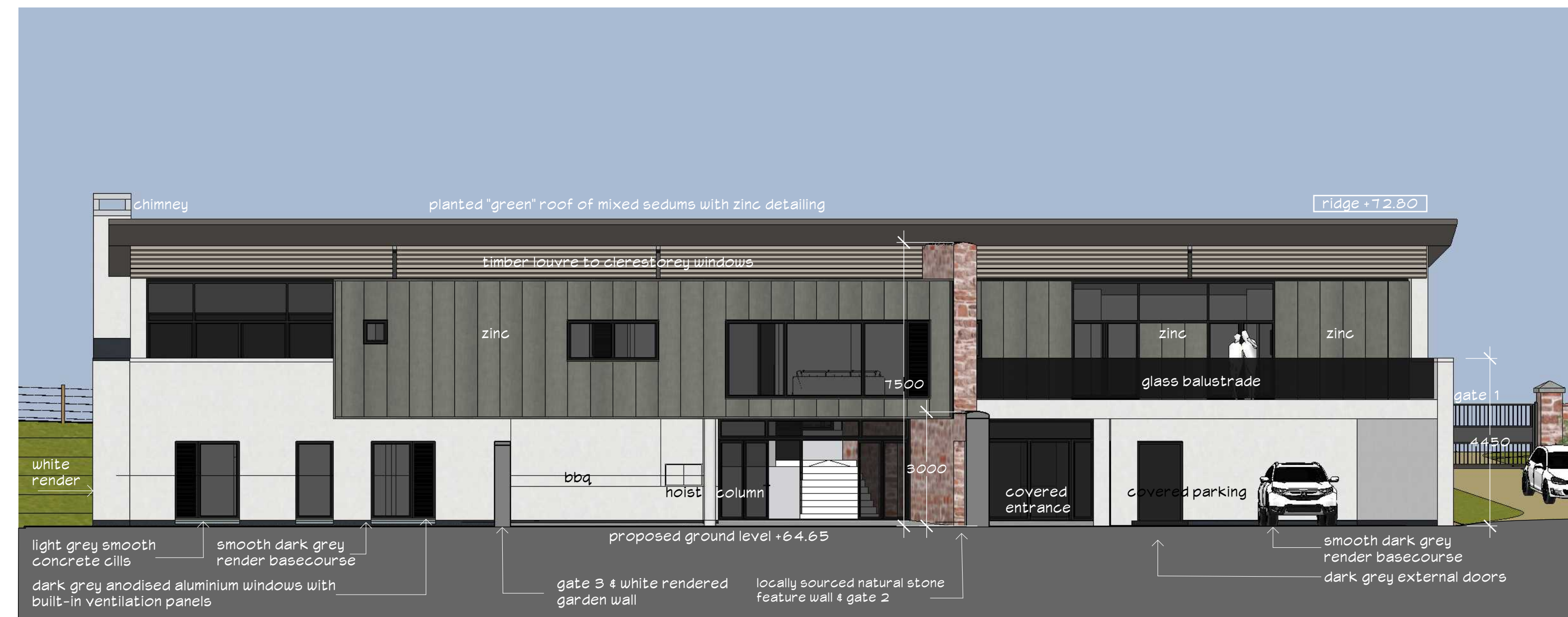
Proposed south elevation- 1:100 @ A 1
