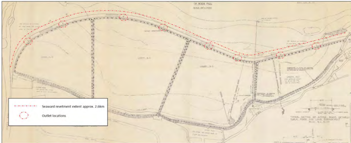
Figure 3 - Location of seaward revetment [Extract taken from Drawing Number 35672c General Layout & Typical Cross Sections of Embankments, (James Williamson and Partners, 1963)]
