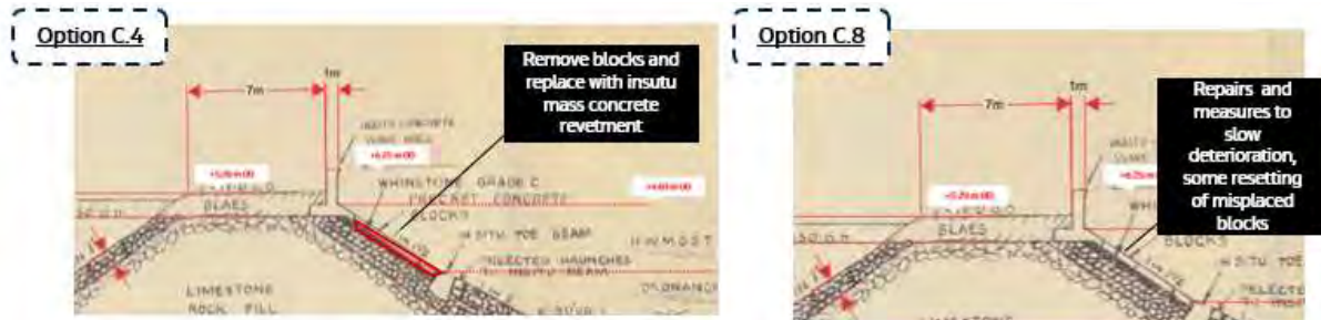
Figure 9 - (C.) Hexagonal Units Short Listed Option C.4 and C.8 indicative sketch
