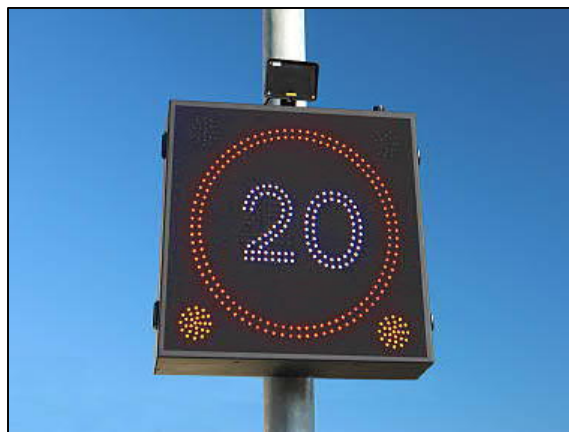
Figure 8.4 - Speed reactive signs
