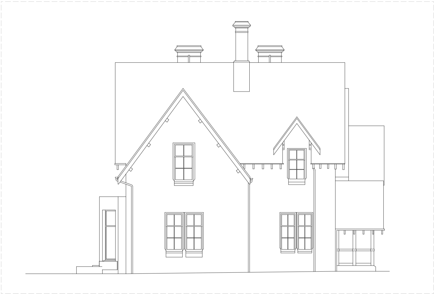
Existing East Elevation 1:100
