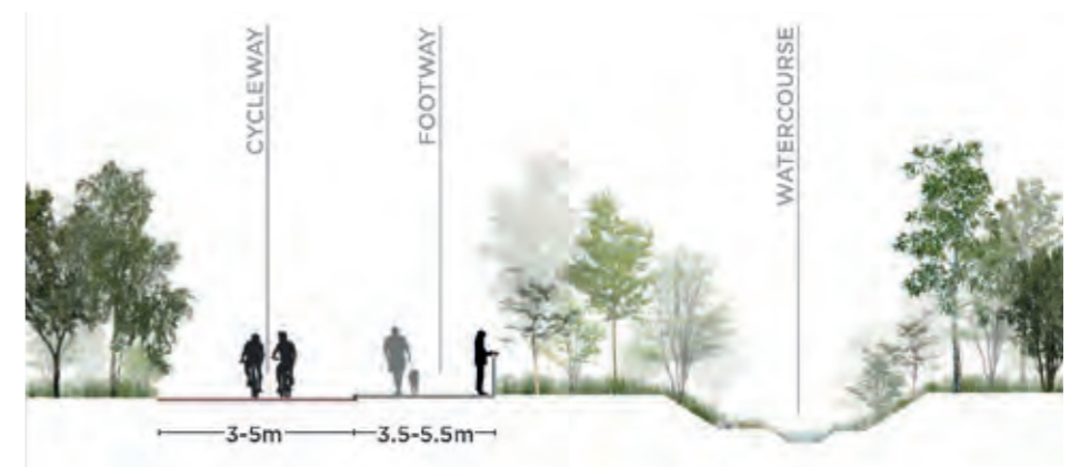
Typical restored watercourse section with new planting and active travel corridor
