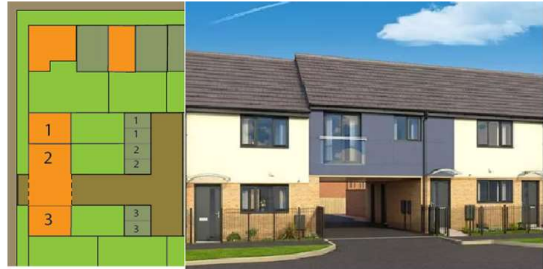
An example of a small rear parking court with a coach house ("Bridge over unit") that makes a clearer definition that the rear court is private.
