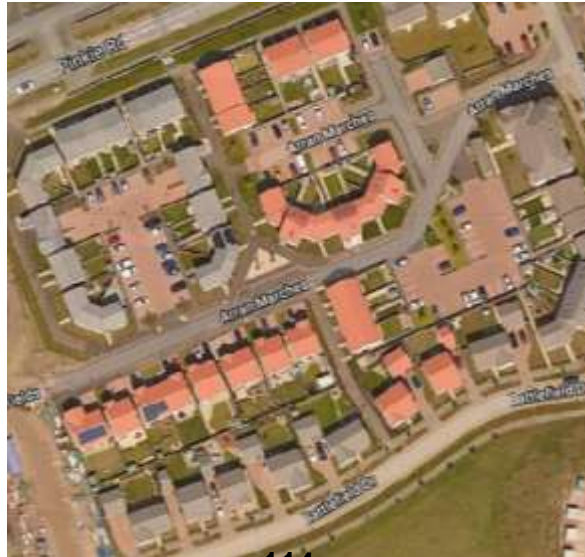
Pinkie Farm, Musselburgh – the layout of new streets responds the existing context and includes longer streets on an east-west axis which helps to maximise solar gain. New dwellings should be constructed to take advantage of sunlight to provide a pleasant living environment and to maximise solar gain. This can be achieved by positioning main living areas, conservatories and rear gardens to generally face south, south-east or south-west where practicable.
