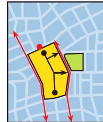
The typical cul-de-sac response creates an introverted layout which fails to integrate with its surroundings
