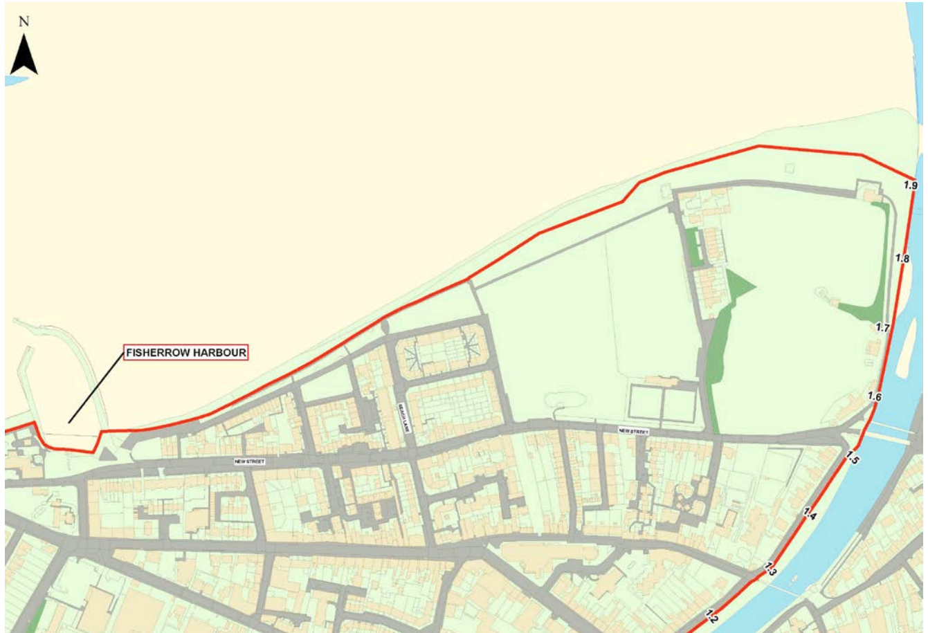
Figure 3.21 Potential alignment of coastal direct defences from River Esk Estuary to Fisherrow Harbour.
