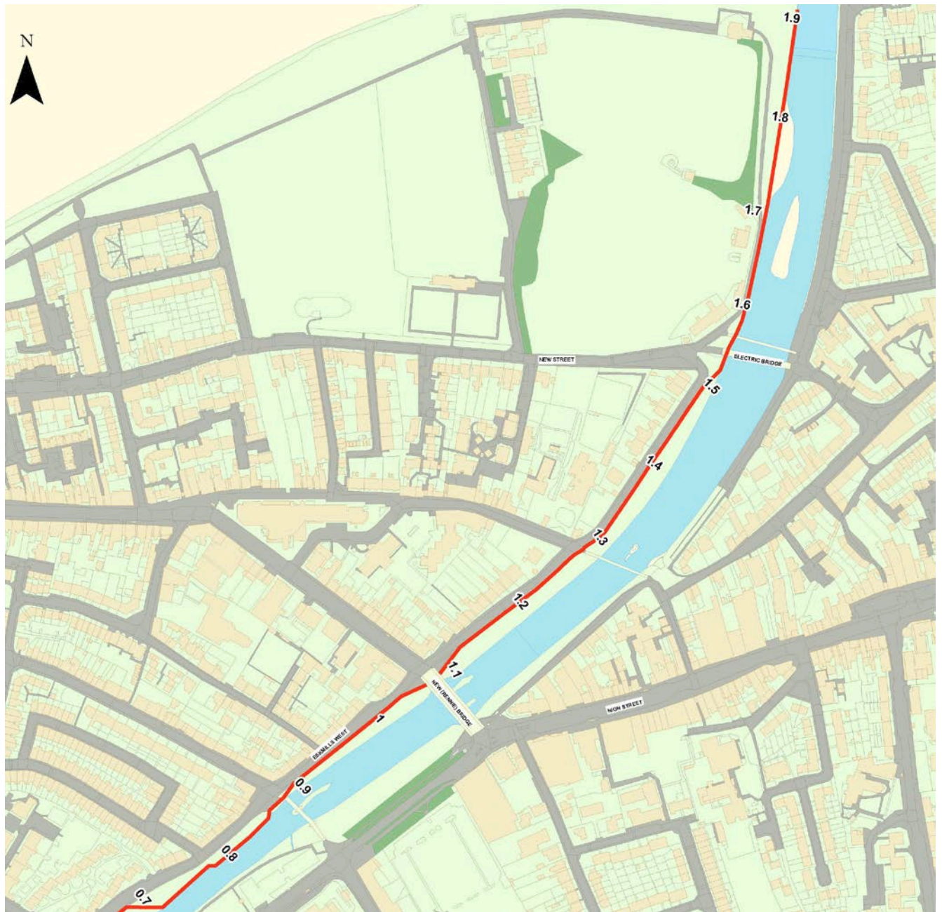
Figure 3.19: Potential alignment of direct defences at Cell 2.
