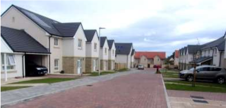
Cross gable roof together with changes in height help to improve the street character.
