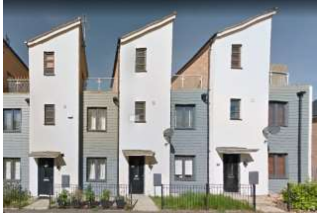
The design of these town houses provides roof terraces whilst protecting the privacy of their occupiers. Selkirk Drive Milton Keynes. Source: GoogleStreet
