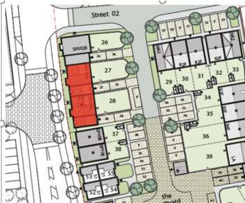
A hypothetical site layout where the rear access to garages and in-curtilage parking is via a short service lane.
