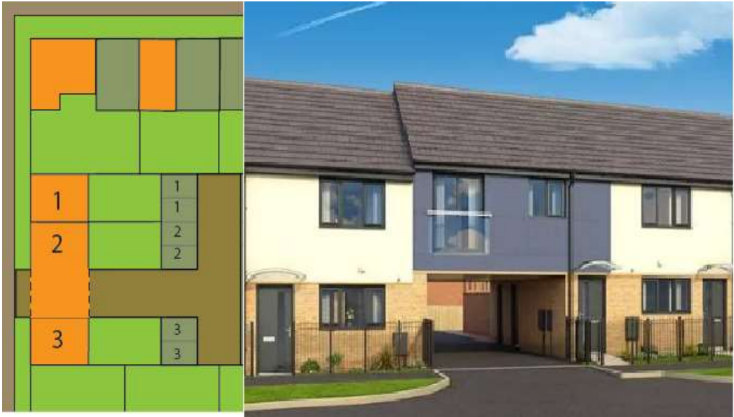
An example of a small rear parking court with a coach house (“Bridge over unit”) that makes a clearer definition that the rear court is private.
