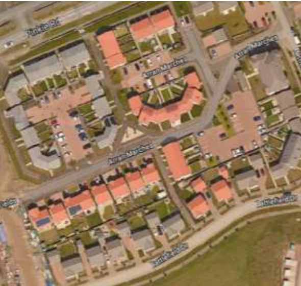
Pinkie Farm, Musselburgh – the layout of new streets responds the existing context and includes longer streets on an east-west axis which helps to maximise solar gain. New dwellings should be constructed to take advantage of sunlight to provide a pleasant living environment and to maximise solar gain. This can be achieved by positioning main living areas, conservatories and rear gardens to generally face south, south-east or south-west where practicable. North-facing gardens may need to be longer than south-facing gardens.
