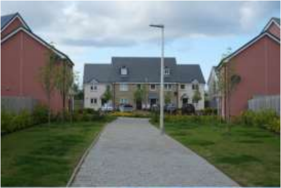
Pedestrian/cycle paths can further improve permeability within new residential developments. These segregated paths must be appropriately overlooked from nearby residential properties and should be additional to any footpaths that are required as part of the street network.
