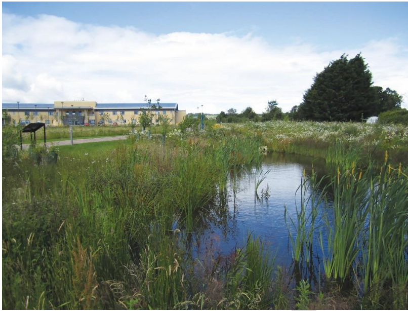
Above: barrier planting prevents access to standing water.
