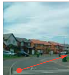
Example illustrates that bend and horizontal carriageway displacement is not combined with a vertical measure to obscure the long sightline. The driver still has long sightline, encouraging higher vehicle speed.
