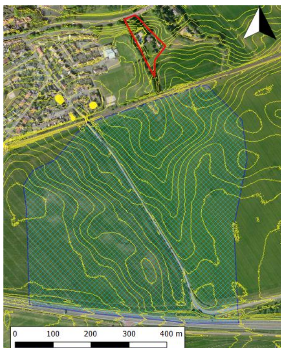
Figure 5 - Overland Flow Catchment
