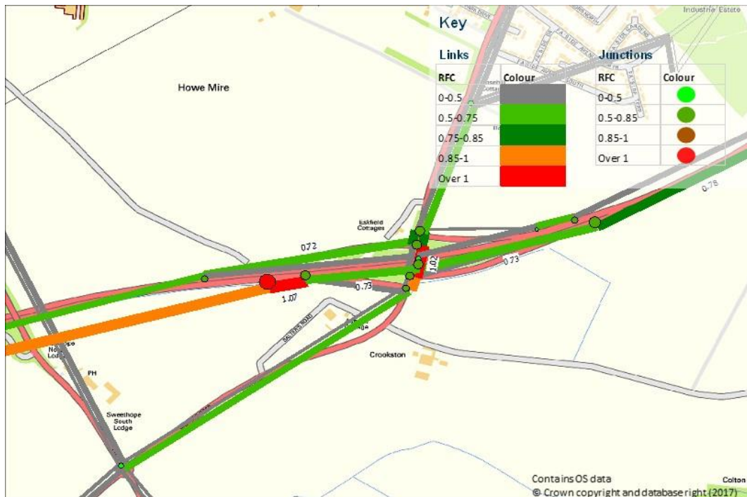
Figure A.28 RFC at A1 Salters Rd Interchange – LDP With Mitigation Scenario – AM Peak Hour
