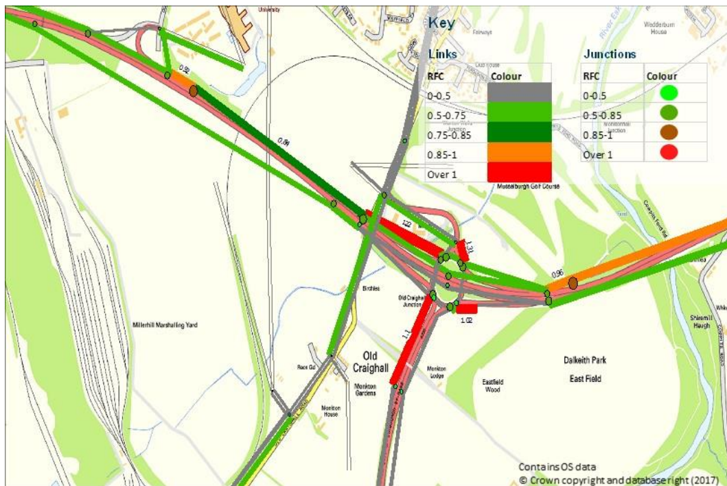
Figure A.23 RFC at Old Craighall– LDP Without Mitigation Scenario – PM Peak Hour
