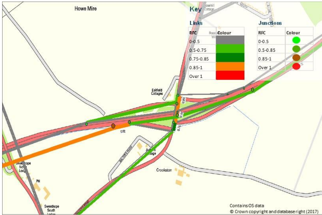
Figure A.16 RFC at A1 Salters Rd Interchange – Without LDP Scenario – AM Peak Hour
