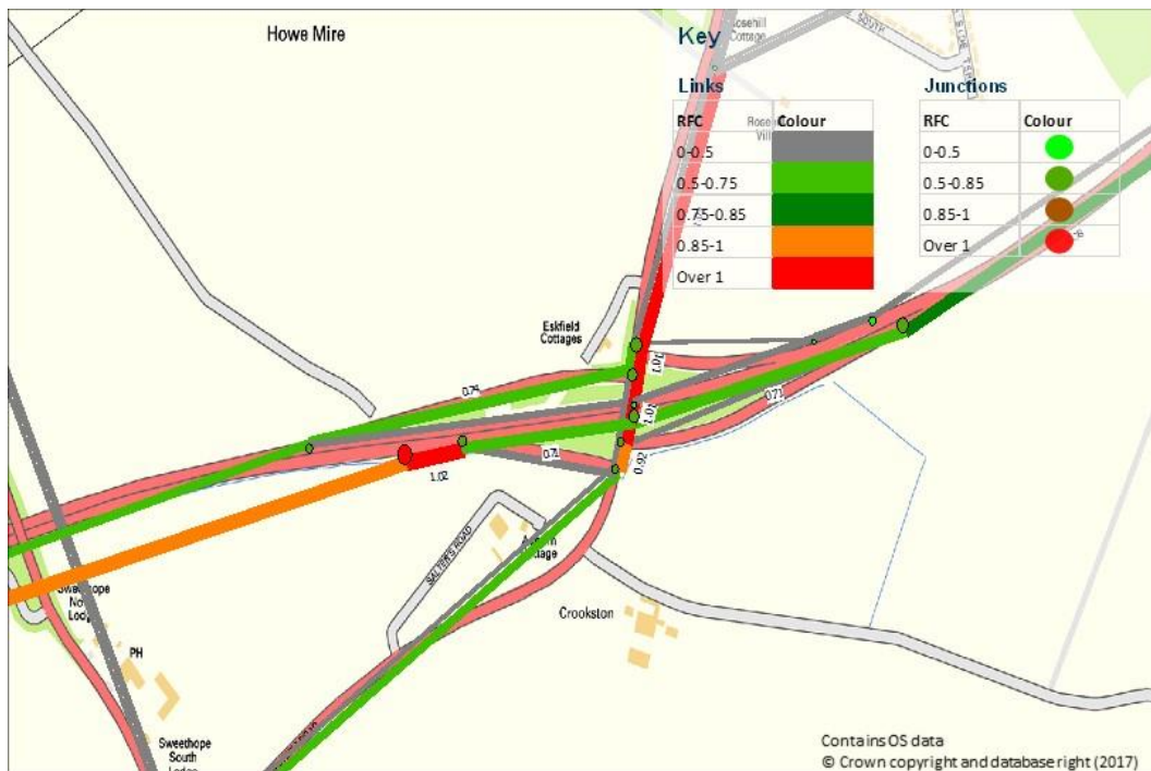
Figure A.17 RFC at A1 Salters Rd Interchange – LDP Without Mitigation Scenario – PM Peak Hour
