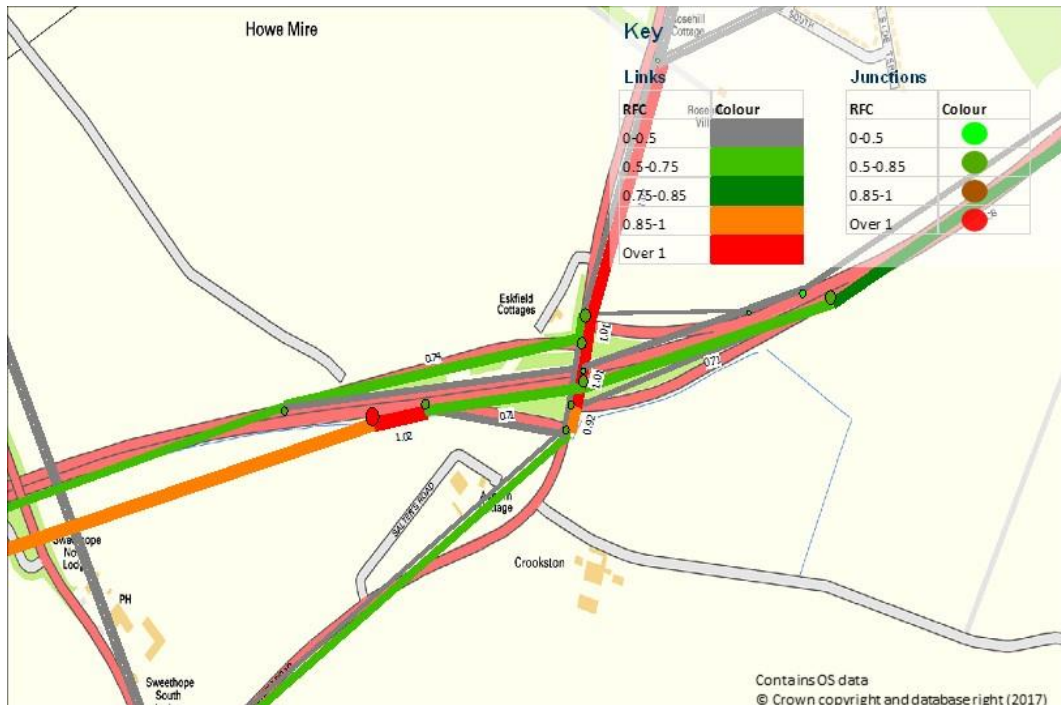
Figure A.27 RFC at A1 Salters Rd Interchange – LDP Without Mitigation Scenario – AM Peak Hour
