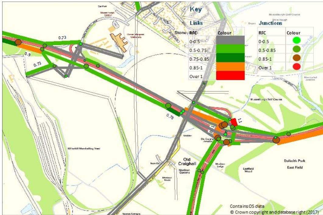
Figure A.22 RFC at Old Craighall – LDP With Mitigation Scenario – AM Peak Hour
