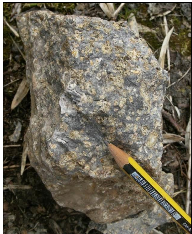
Photo ELC_12 P8: Close up of the porphyritic trachyte which was extracted from the quarry and used to construct many of Haddington's stone buildings. © BGS, NERC.
