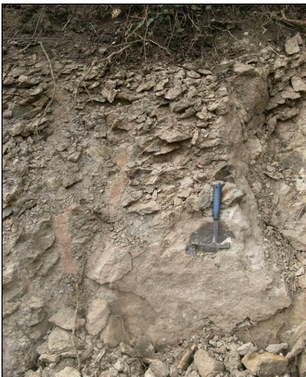
Photo ELC_12 P7: Detail of the uppermost part of the quarry face showing the increasingly weathered nature of the igneous rocks towards the natural surface. © BGS, NERC.
