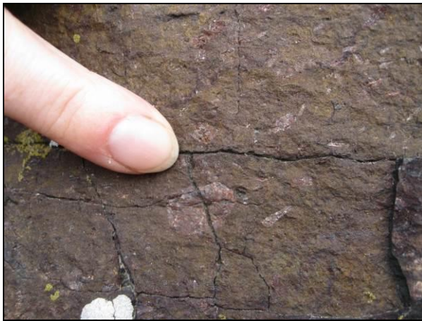
Photo ELC_5 P4: The grey-red basalt protecting the north-west wall of North Berwick harbour contains abundant mineral crystals, namely plagioclase feldspar phenocrysts (<5 mm in size) with occasional 1 cm euhedral labradorite feldspar phenocrysts set in a fine grained groundmass. Occasional <1 mm sized phenocrysts of pyroxene and olivine pseudomorphs can be identified within the face, such as the large crystal being pointed to in the photo. The presence of large crystals set in a fine grained groundmass are indicative of two phases of cooling in this lava flow – a slow, initial cooling forming larger crystals (probably within the magma chamber) and a fast, rapid cooling during eruption which formed the fine grained groundmass. © BGS, NERC.
