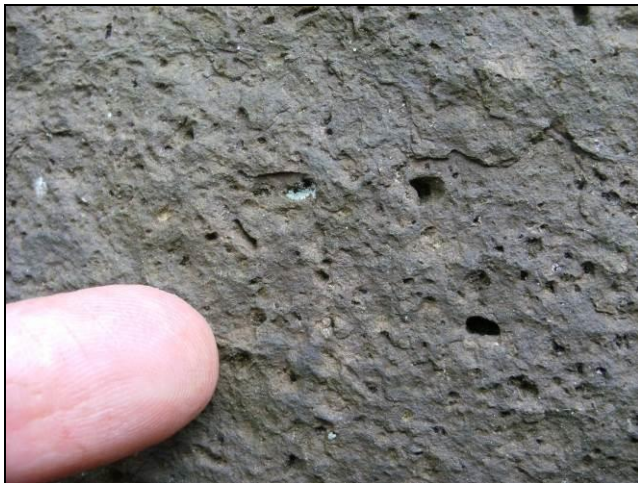
Photo ELC_10 P5: Weathered out feldspars and vesicles (formed by gas bubbles within the laval) give the trachyte a pockmarked appearance in places. © BGS, NERC.
