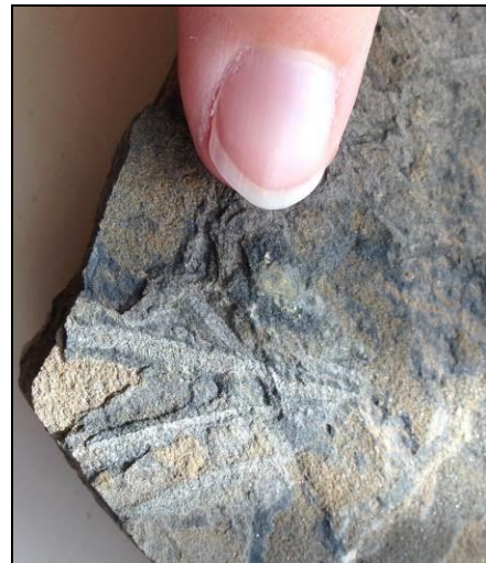
Photo ELC_1 P3: Hand specimen from the site reveals a black shale layer containing abundant graptolite fossils. Graptolites are one of the characteristic fossils used to help define the stratigraphy of the Ordovician and Silurian successions, and have been used to define 'biozones' throughout the strata, aiding geologists in dating the sequence. Graptolites, marine colonial organisms, lived from the Upper Cambrian to the Lower Carboniferous. © BGS, NERC.
