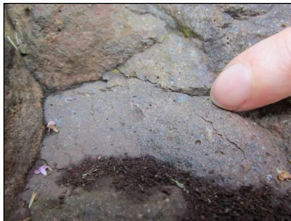
Photo ELC_9 P3: Detail of the macroporphyrritic basalt, bearing phenocrysts of pseudomorphs after olivine, pyroxene, and feldspar. The rock shown is also partially vesicular – the small, spherical hollows are the remnants of what would have been gas bubbles that became trapped in the basalt as it cooled. © BGS, NERC.
