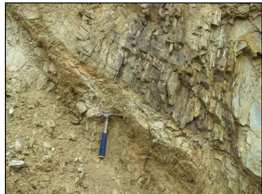
Photo ELC_1 P5: A 10cm wide fault zone is exposed at the north end of the east wall, composed chiefly of brecciated clasts of the surrounding siltstone. Photo taken looking west. © BGS, NERC.
