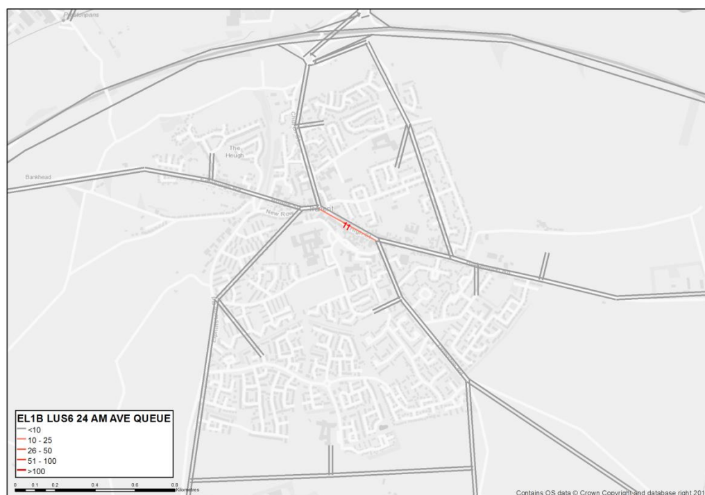
Figure 5.8 Average Queues (PCUs) in Tranent Town Centre – With LDP Scenario – AM Peak Hour
