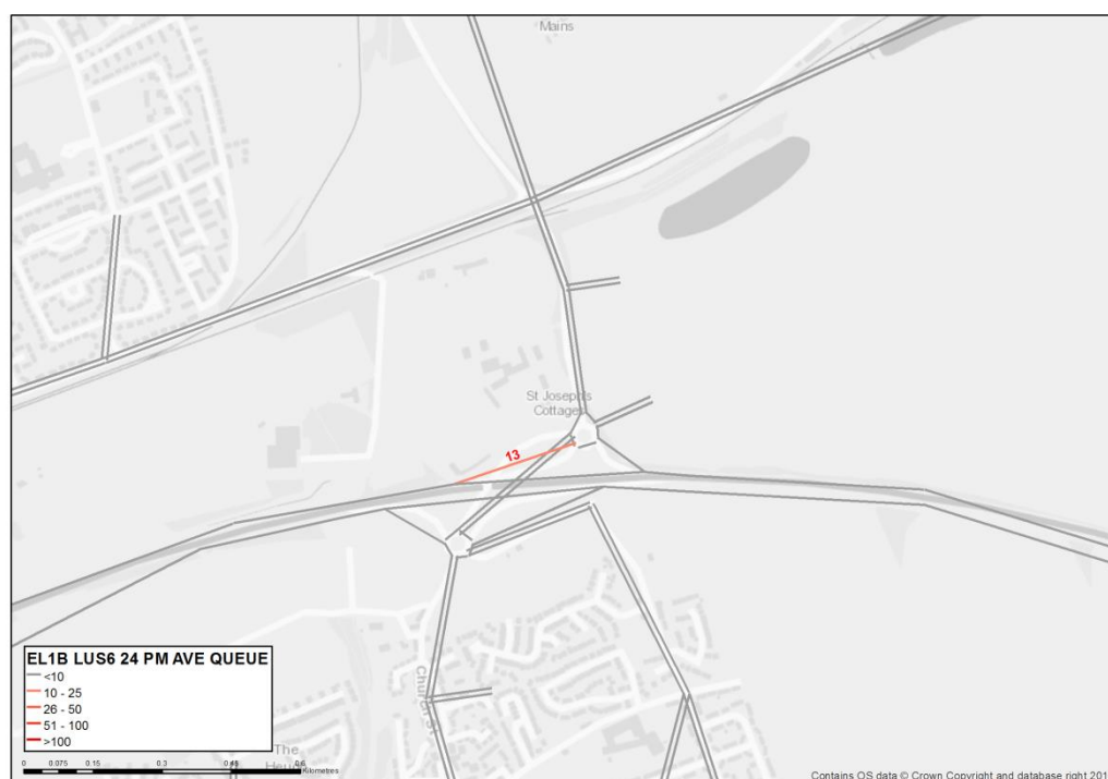
Figure 5.5 Average Queues (PCUs) at A1 Bankton Junction – With LDP Scenario – PM Peak Hour
