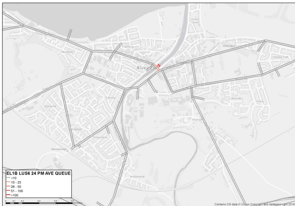
Figure 5.7 Average Queues (PCUs) in Musselburgh Town Centre – With LDP Scenario – PM Peak Hour
