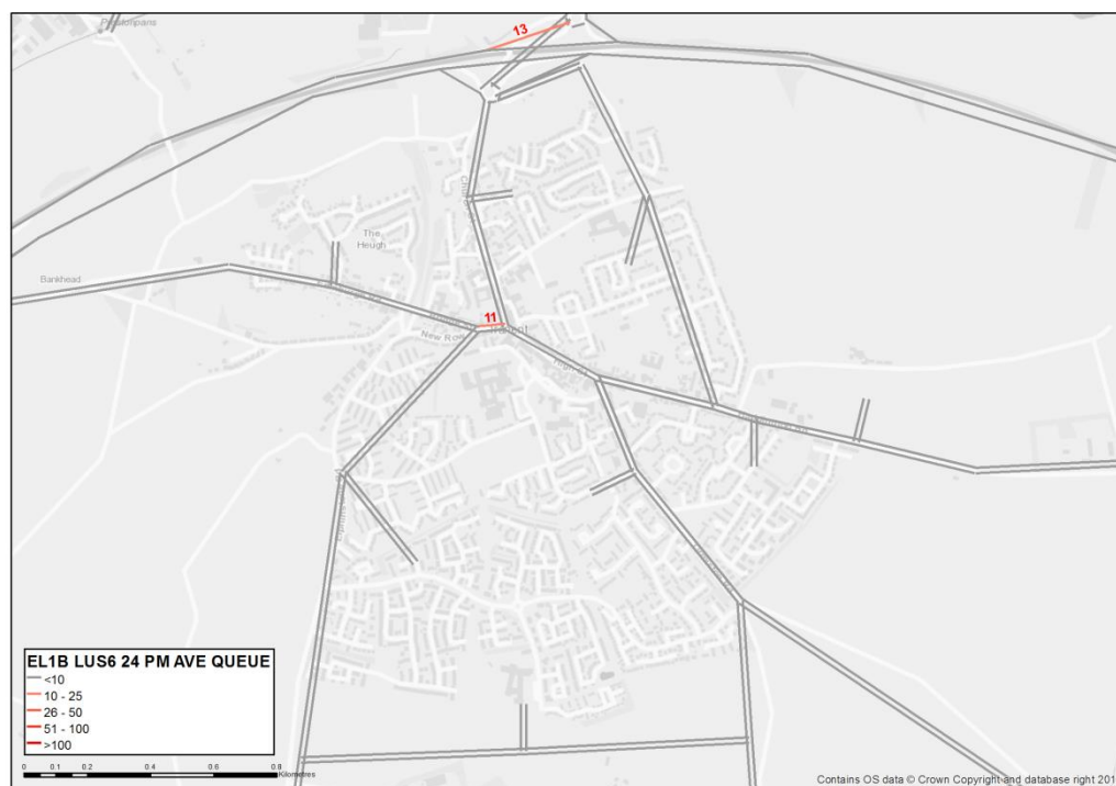
Figure 5.9 Average Queues (PCUs) in Tranent Town Centre – With LDP Scenario – PM Peak Hour
