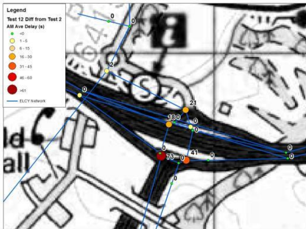
Figure 90. Test 12 vs Test 2 Junction Delay – Old Craighall
