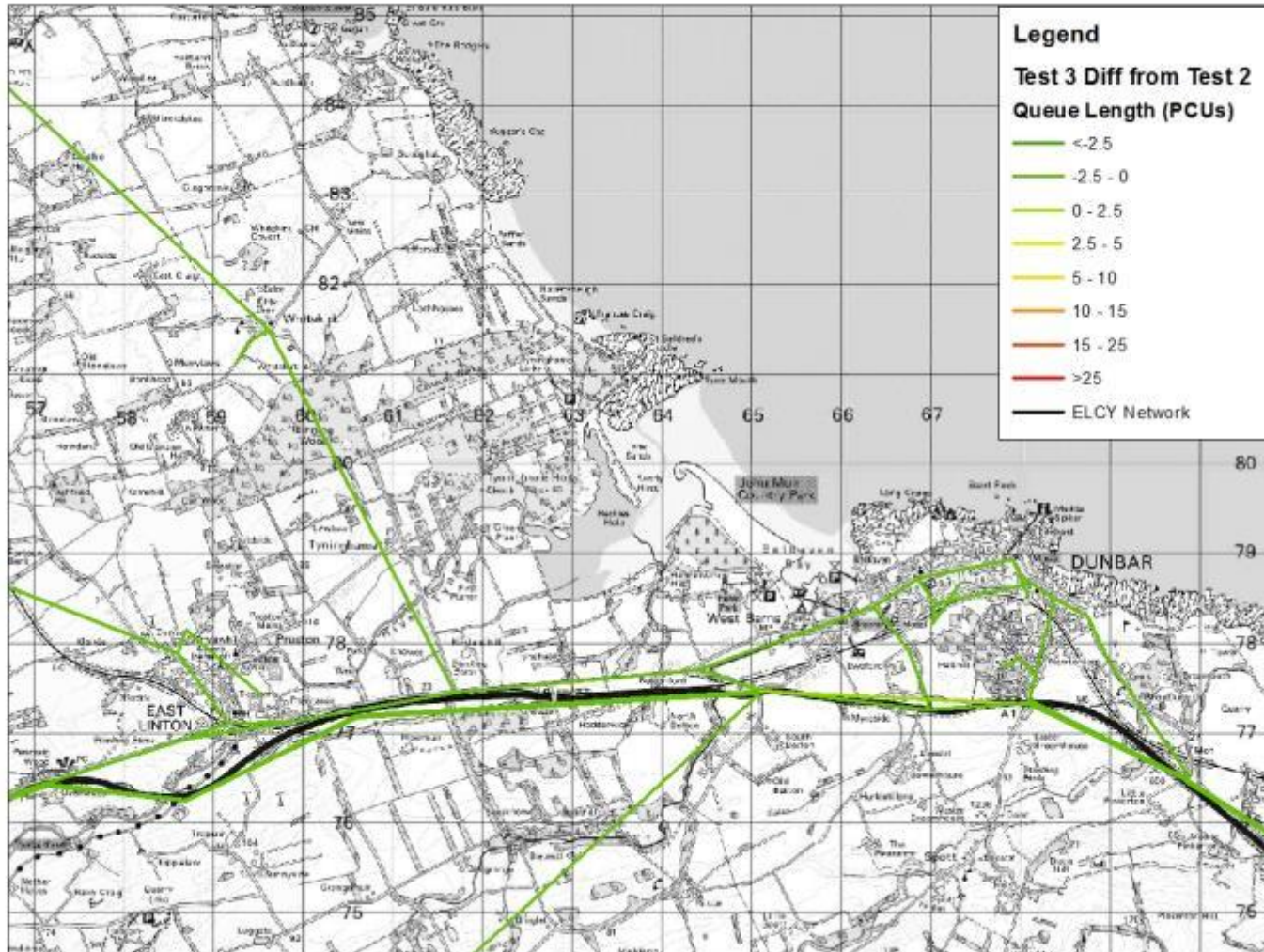
Figure 26. Test 3 vs Test 2 Queue Lengths – East
