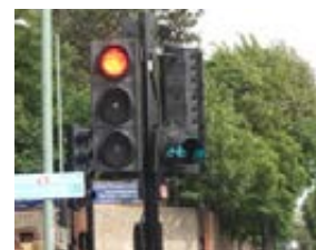
Green cycle pre-signal gives 5 seconds head start for cyclists, Examples in Brighton, York and Cambridge (requires authorisation)
