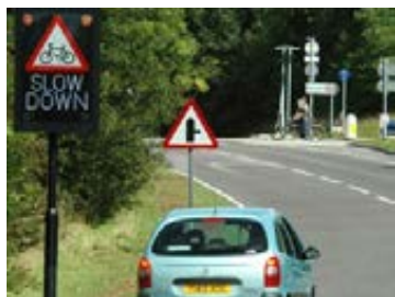
Cycle activated warning at crossing, Leicestershire
