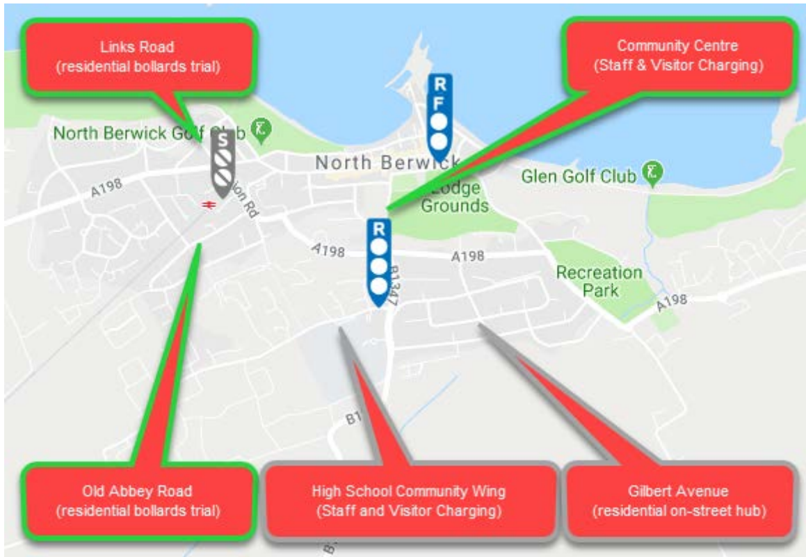
Figure 11: Proposals additional chargepoints in North Berwick
